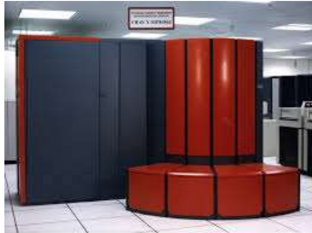
Cray Y/MP 8/432 4 * 200 MHz 64bit 256MB RAM 20GB Disk
